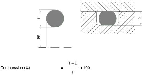
Seat width D according to the cord diameter T and the % compression
