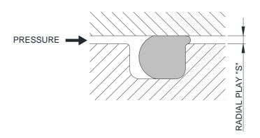
The acceptable radial play "S" between the sealing surfaces dipends on the pressure of the system, the cord section and the O-Ring hardness.
