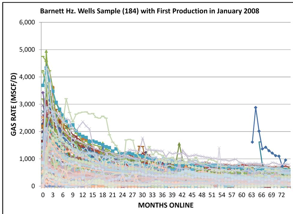
Figure 3—Example of horizontal wells' shale gas production data.
