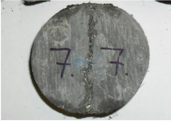
Figure 3. Photo of a partially damaged specimen in split test (Bragov et al. 2012).
